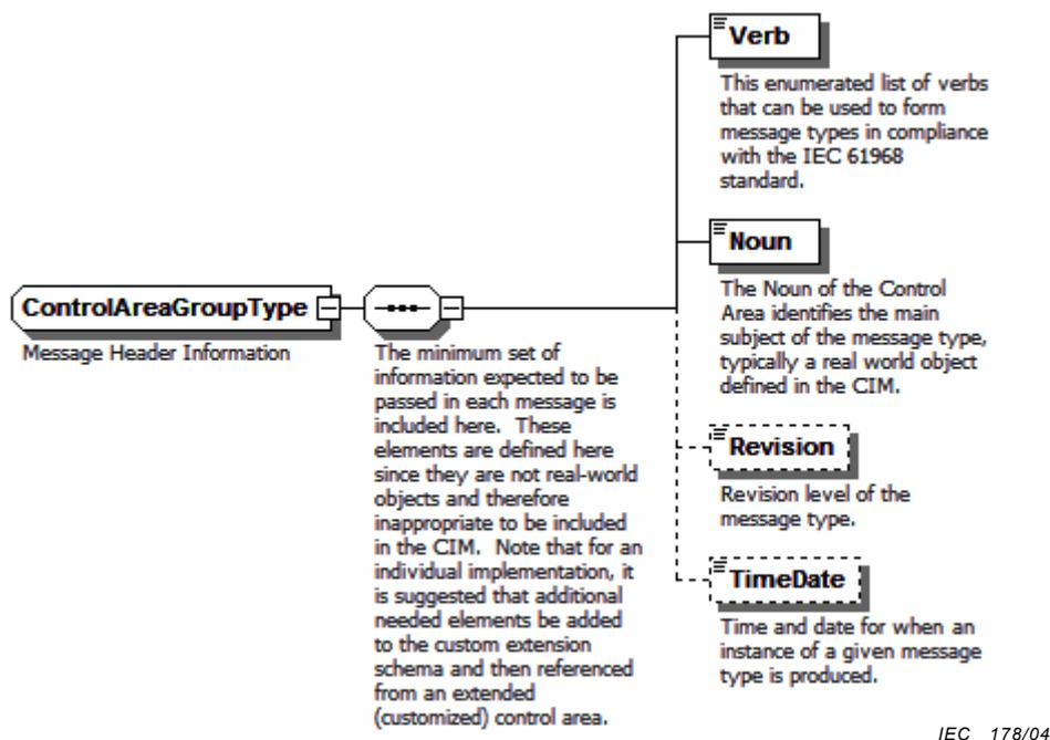
**Figure 3 – Example (informative) of a control area used for all message types**
